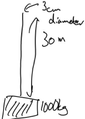
$$\Delta L = \frac{FL}{A\gamma} = \frac{(1000 \text{ kg})(9.8 \text{ m/s}^2)(30 \text{ m})}{\pi(1.5 \times 10^{-2} \text{ m})^2 (2 \times 10^{11} \text{ N/m}^2)} = 2.1 \times 10^{-3} \text{ m} \\ = 2.1 \text{ mm}$$
